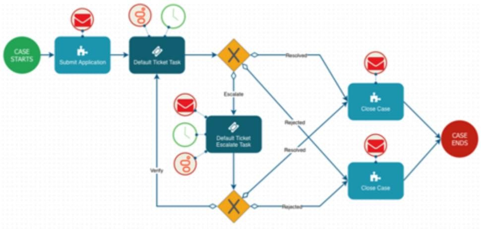
On each task (Dark Blue) a SLA can be set to meet your business' SLA's. (Depicted by the green clock icon). Based on the Employees wrap-up (completion code) on the first task (Resolved, rejected to Escalate) the next step is taken. This could be automated closure with sending the customer a confirmation email/SMS/Notification with the outcome, or a new task send to an Escalation group.
