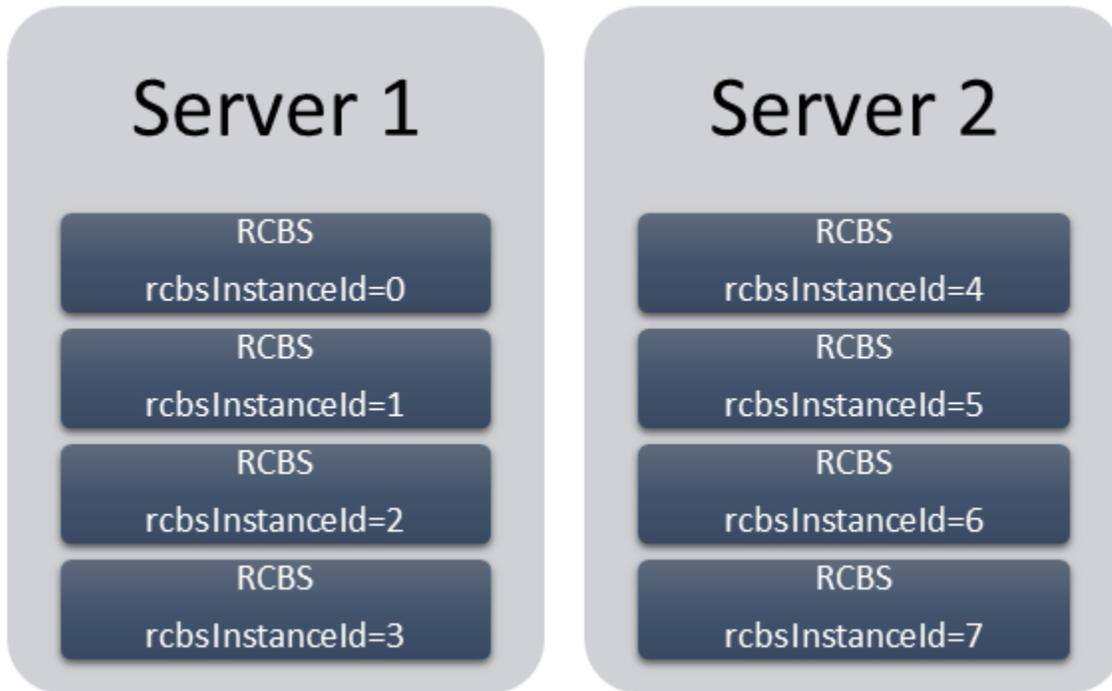
In the above image, eight instances of RCBS spread between two servers. Here, the value of **totalRcbsInstances** is 8 in all the instances.
