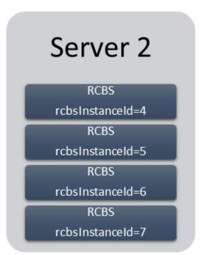
In the above image, eight instances of RCBS spread between two servers. Here, the value of **totalRcbsInstances** is 8 in all the instances.
