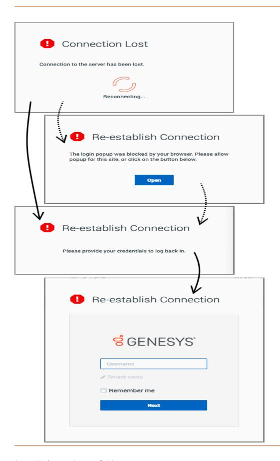
Workspace is designed to handle system disconnections. If the server that directs interactions to you becomes disabled or disconnected for some reason Workspace automatically tries to connect you to a backup server so that you can keep serving your customers with minimal interruption. If a connection loss occurs, you are instantly informed by the **Connection Lost** message. Workspace immediately tries to reconnect you.
