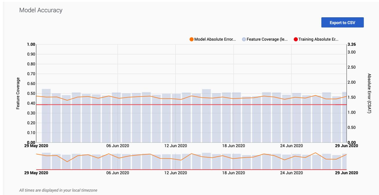
The Model Accuracy graph shows the mean absolute error value, indicating the difference over time between the results the model predicts and the actual outcomes. This value, and how to interpret it, varies depending on the type of key performance indicator (KPI) your model optimizes.
