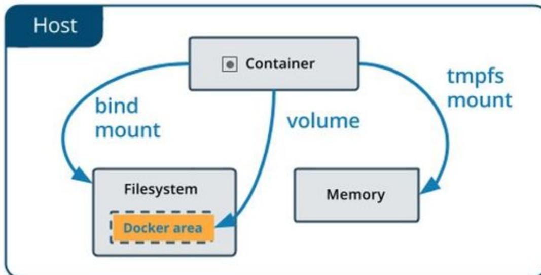
If your container generates non-persistent state data, consider using a **tmpfs mount** to avoid storing the data anywhere permanently, and to increase the container's performance by avoiding writing into the container's writable layer. Volumes use rprivate bind propagation, and bind propagation is not configurable for volumes.
