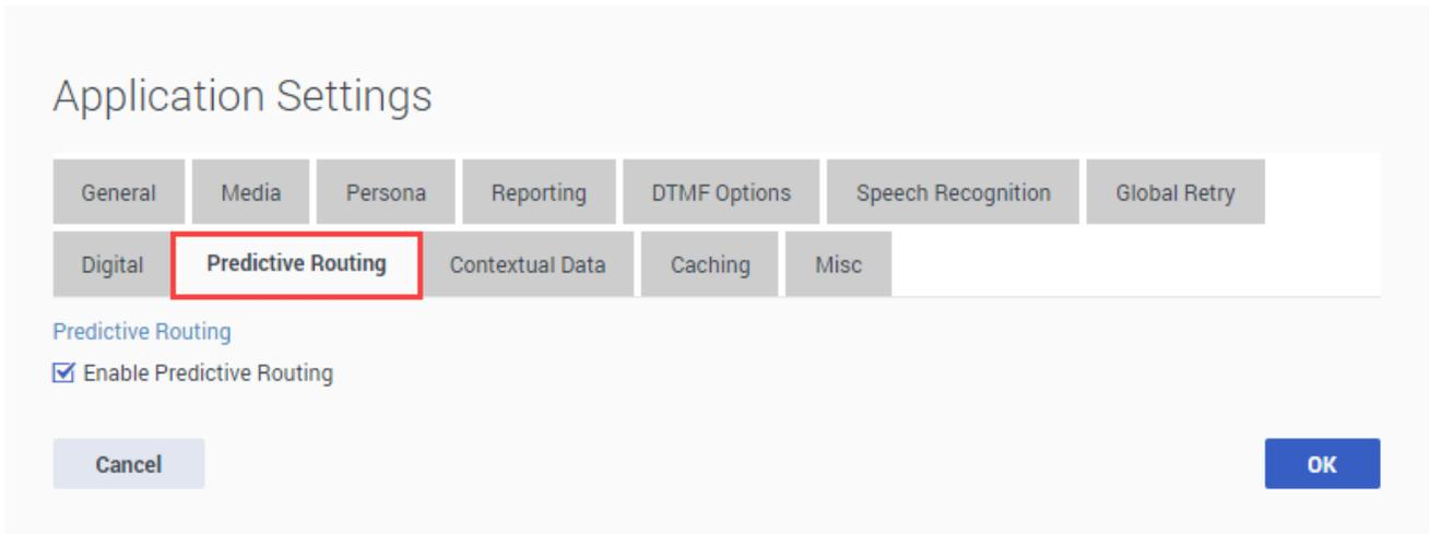
Select this option to enable support for predictive routing (as required for the Predictive Routing block).
