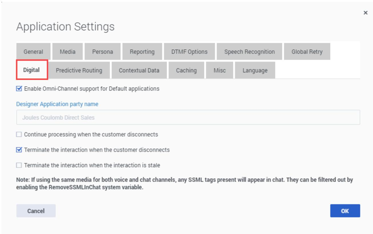
The **Digital** tab of the application settings allows you to enable omni-channel support for Default applications. When enabled, it allows your application to handle both voice and chat interactions.
