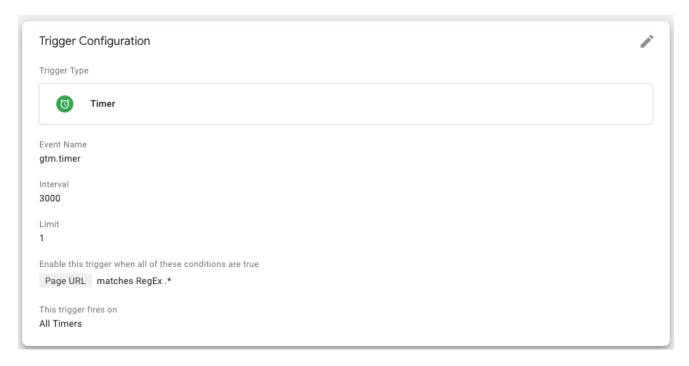
This example shows how to define a trigger to track whether a webpage remains open for 3 seconds.
